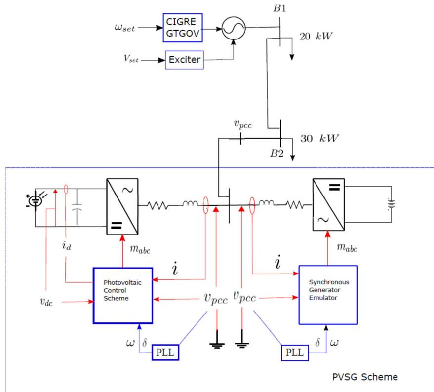
Fig. 8. Microgrid Test System for 40kVA PVSG system.
