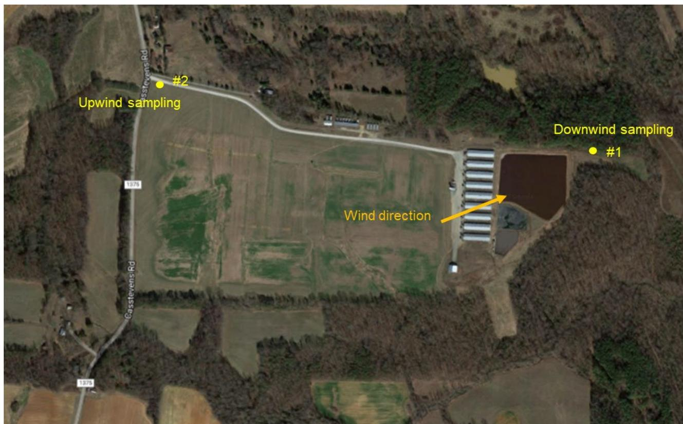
Figure 5. Aerial view of the facility and location of the monitoring points for odor for the March 14, 2019 sampling. The location was about 50 yards downwind of the little hunting hut. The arrows indicate the prevailing wind direction the day of the sampling.
