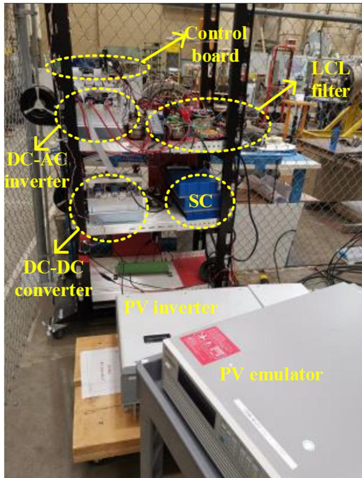
Fig. 5. Experiment setup.
