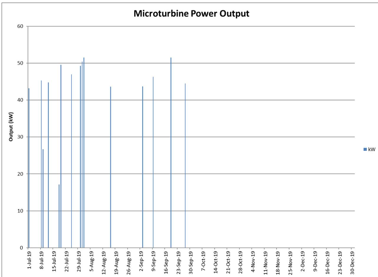
Figure 2. Microturbine Output (kW) (July 1, 2019 -December 31, 2019)
