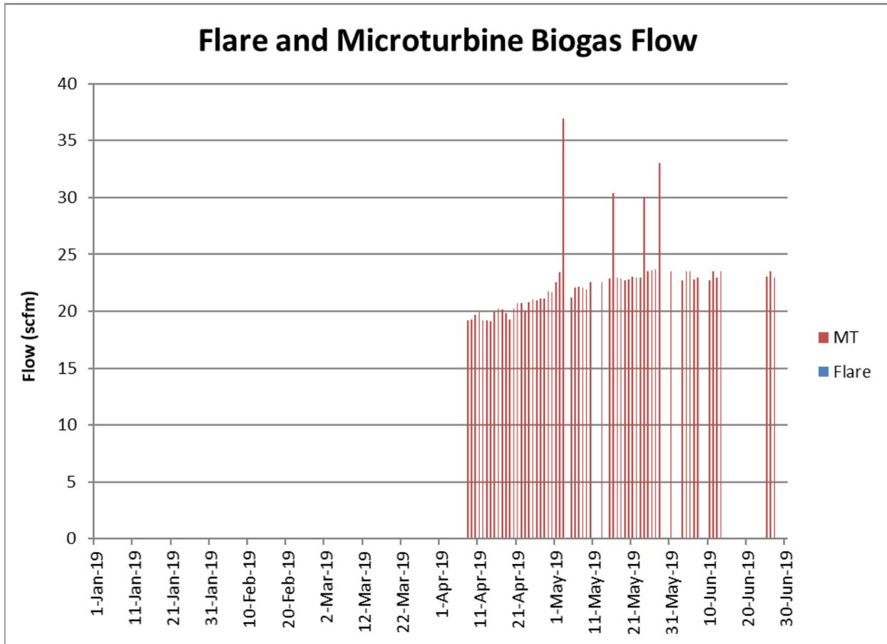
Figure 2. Measured Biogas Flow and Flare Usage (SCFM)
