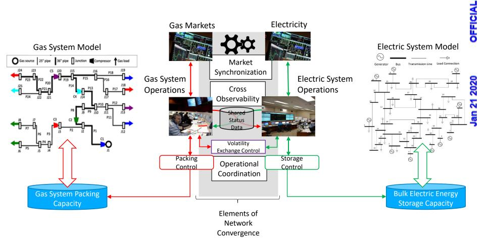
These two connected systems have different flow rate requirements. Storage (on both sides) can resolve the mismatch.
