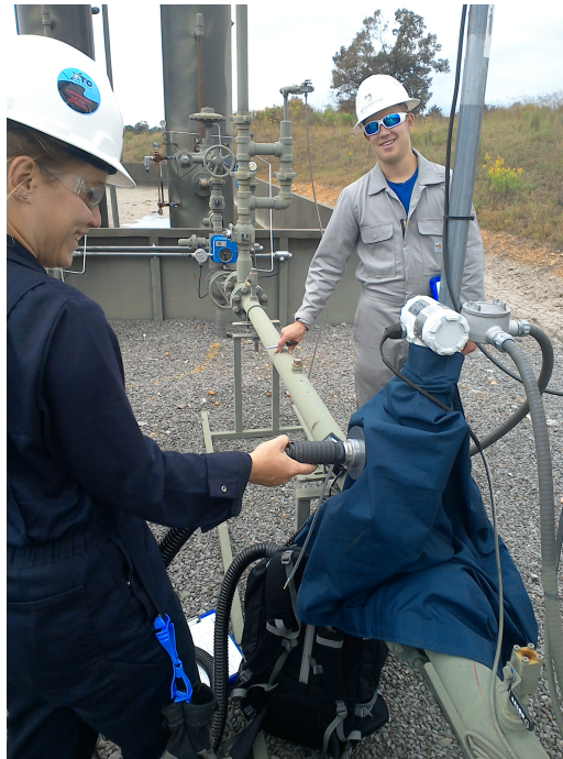
Figure 1: Easily accessible high-flow measurement using bag attachment.
