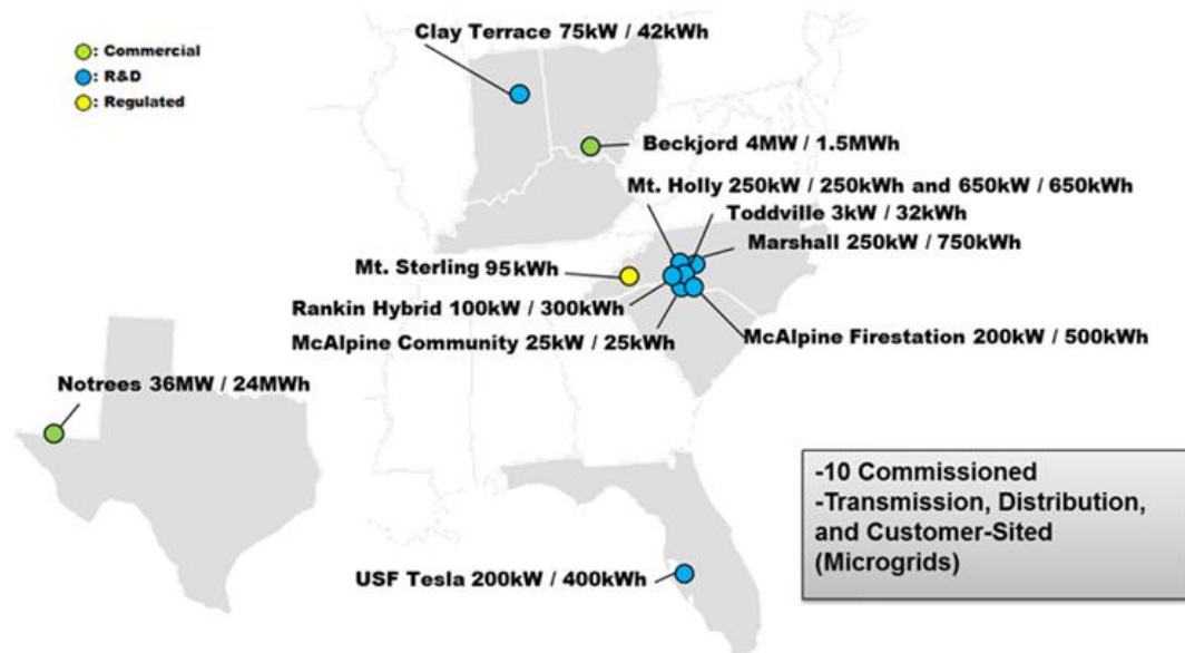
Figure F-5: Existing, Operational Duke Energy Battery Storage Assets
