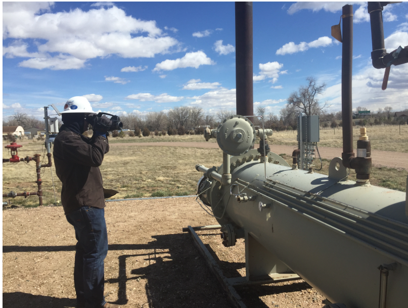
Figure 1: Optical gas imaging (OGI) will be used as the primary emission screening tool.
