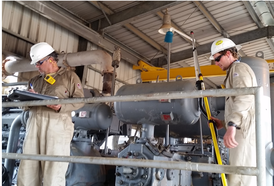
Figure 2: Using an adapter pole to enable high-flow measurement of a hard-to-reach elevated vent above hot, rotating equipment.
