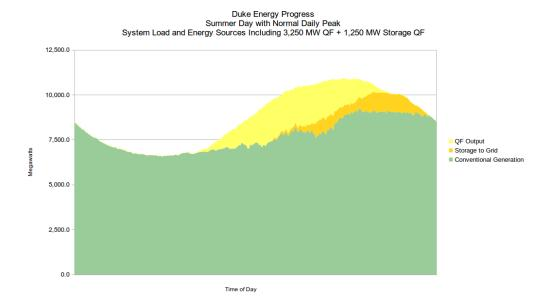
Another important point this example demonstrates: solar + storage can significantly reduce ramping requirements.
