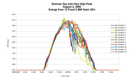
For ease of understanding and discussion, we scaled the NREL data to be equivalent to the output from 12 solar plants that each have 5 MW of capacity – one plant at each location. In contrast, Astrape's simplified solar profiles were developed for just a single location within each grid cell.
