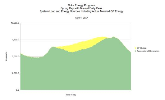
The overall impact of solar production is favorable – displacing conventional generation during much of the day. While the downward ramp in the morning
