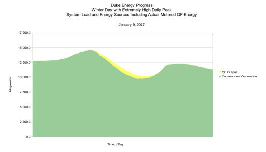
As the day warms up, the demand for electric heating falls, bringing the overall system load down as well. System load drops below 10,500 MW for a couple of hours (starting around 1:30 pm), before climbing to an moving back up to nearly 12,000 MW later in the evening.
