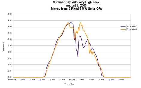
At times during the day, output from both locations moves in the same direction while there are other times a downward fluctuation in one location is offset by an upward fluctuation at the other location. This demonstrates that when solar data from numerous locations is aggregated, it becomes more stable and provides a stronger basis for understanding, forecasting, and responding to solar output variations.
