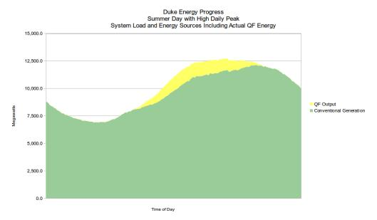
As can be clearly seen in this graph, QF energy is helping to reduce the "net" peak load throughout the middle of the day. As a result, the highest "net" peak is experienced hours after the "gross" peak – at a time when customer demand remains high but solar production is ebbing.
