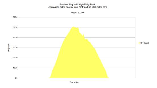
Needless to say, if this much smoothing occurs with such a small data set (just 12 locations in a single grid cell), the output from hundreds of small facilities that are widely dispersed across two states will be even smoother and more easily forecast.
