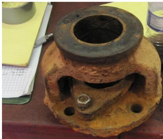
**Turbine Bearing Cradle in poor condition**
