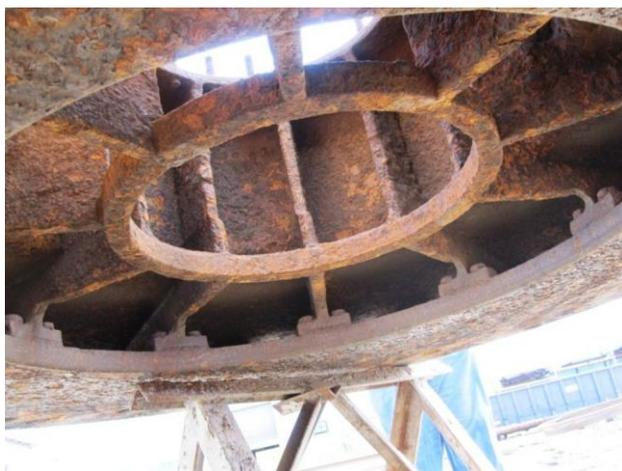
**Headcover damage in cast iron pressure component**
