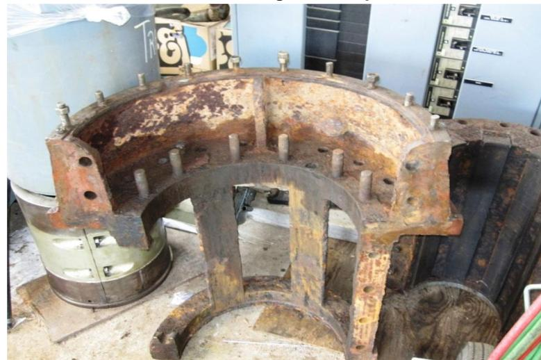
**Turbine bearing in need of rehabilitation**
