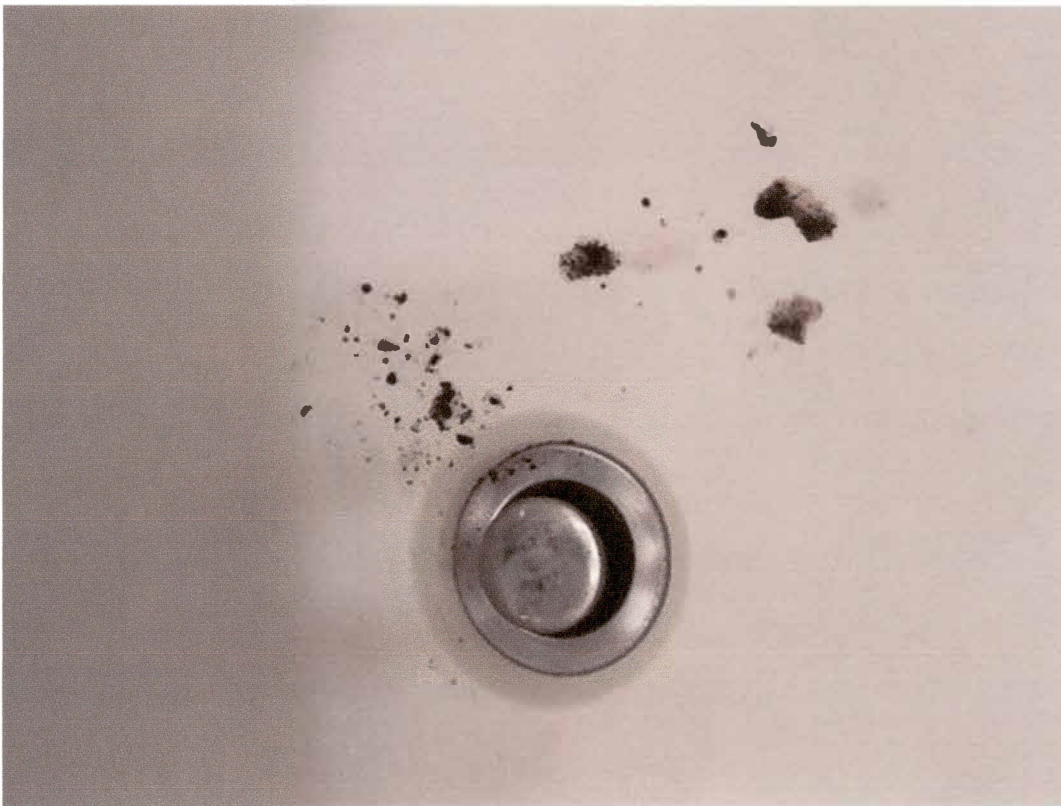
Manganese deposits found in bath tub and bathroom faucet strainer following major sediment contamination episode October 2021 after water system was turned back on following water main repair at Oak Stone and Whitfield roads
