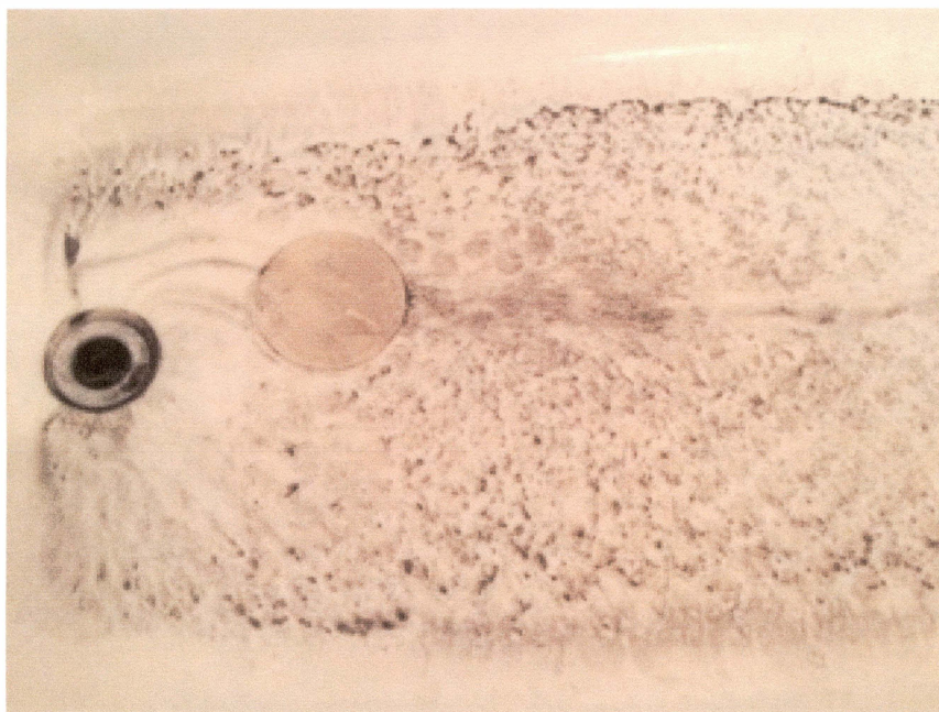
Manganese deposits found in bottom of bath tub after filling tubs as instructed by Aqua storm advisory, February 2021
