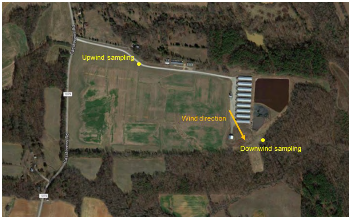
Figure 2. Aerial view of the facility and location of the monitoring points for odor for the July 3 (Q2) sampling. The arrows indicate the prevailing wind direction the day of the sampling.
