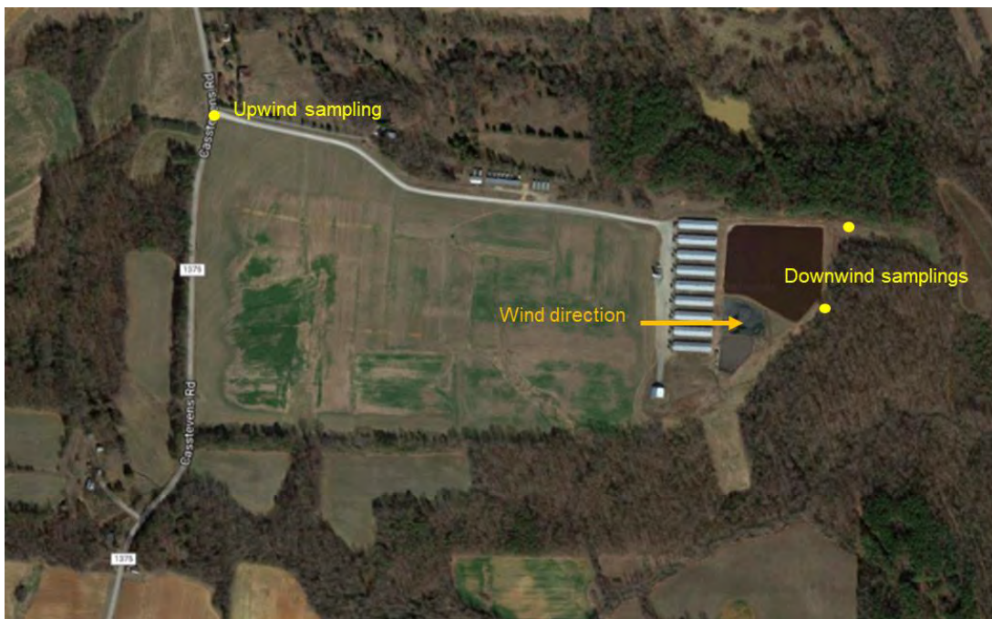
Figure 1. Aerial view of the facility and location of the monitoring points for odor for the March 12, 2020 sampling. The arrows indicate the prevailing wind direction the day of the sampling.
