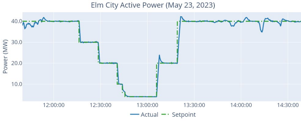
Figure 8 Elm City Active Power Response at Full Reactive Power Absorption
