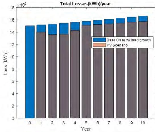
Figure 44: Total losses per year - with and without PV
