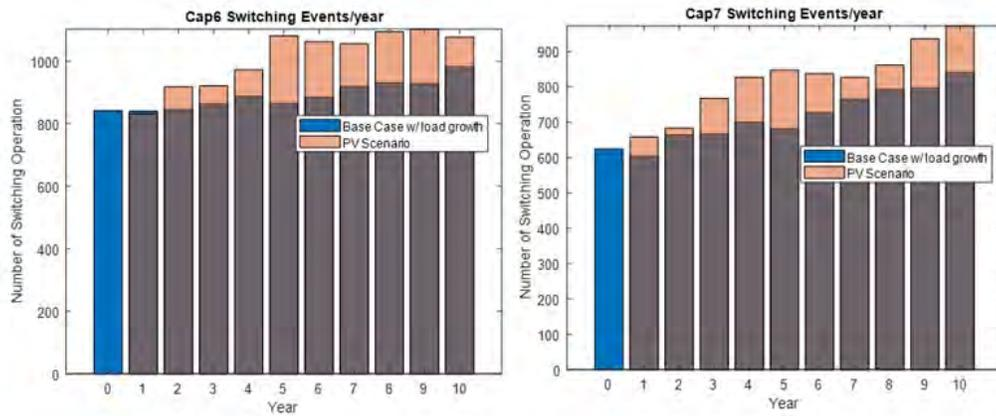
Figure 37: Capacitor switching per year - with and without PV - Left: IEEE 123 PV, Right: IEEE 123 No PV
