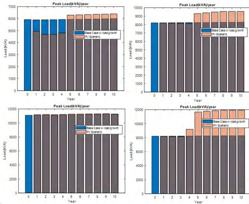
Figure 48: Feeder-wise yearly peak demand - with and without PV, Top Left: J1, Top Right: IEEE 123 PV, Bottom: IEEE 123 No PV
