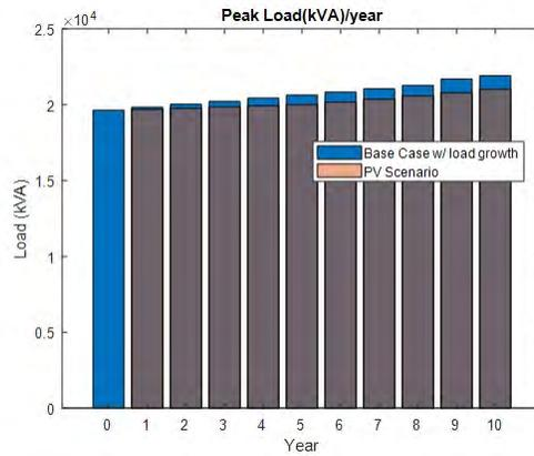
Figure 84: Yearly peak demand at substation - with and without PV
