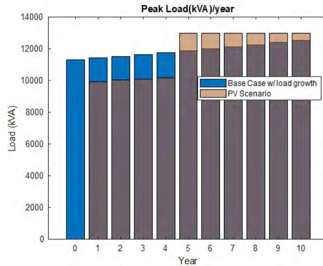
Figure 21: Yearly peak demand at substation - with and without PV
