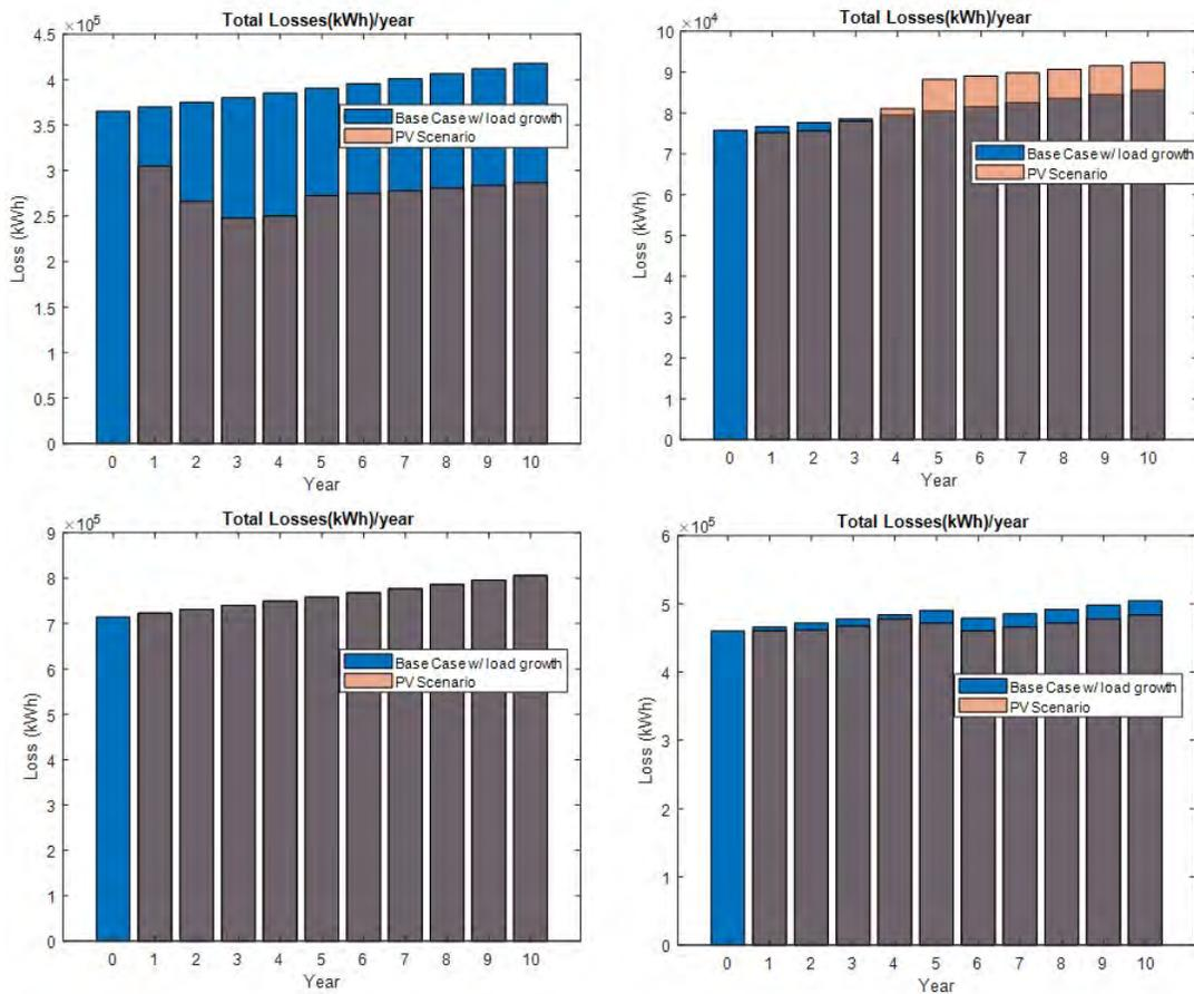
Figure 87: Feeder-wise total losses per year - with and without PV, Top Left: Substation, Top Right: B01, Bottom Left: B02, Bottom Right: B03
