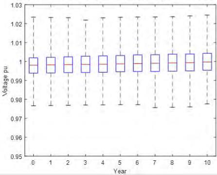
Minimum Circuit Voltage – PV
