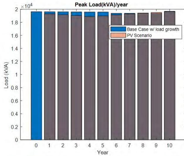
Figure 70: Yearly peak demand at substation - with and without PV
