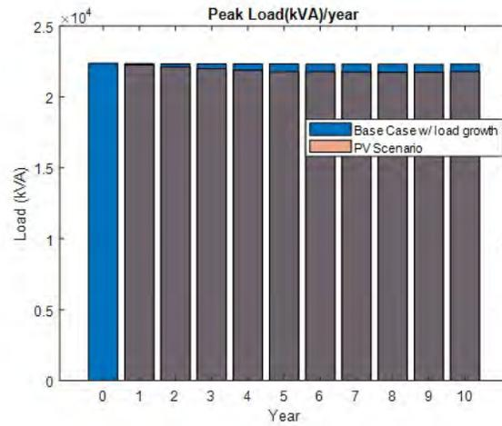
Figure 25: Yearly peak demand at substation - with and without PV
