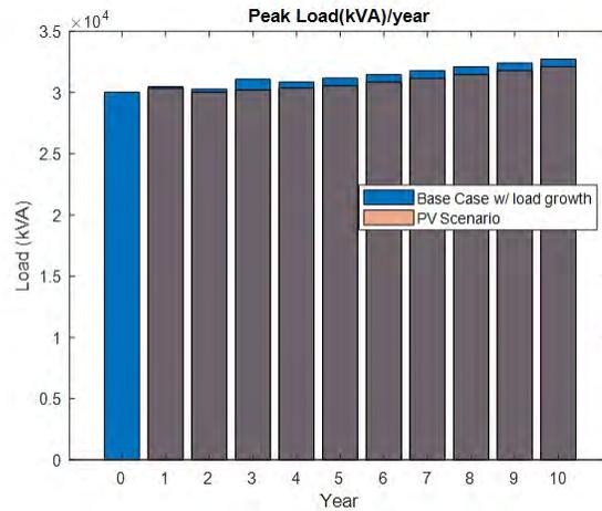
Figure 65: Yearly peak demand at substation - with and without PV
