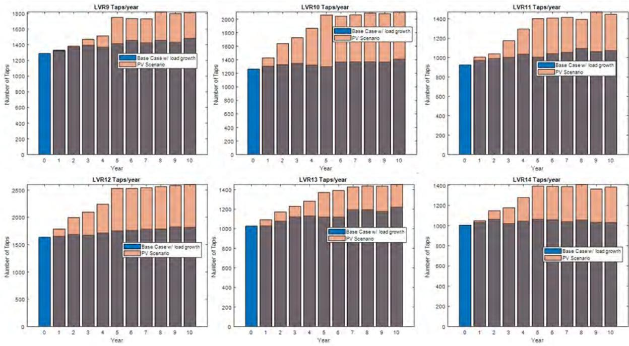
Figure 34: IEEE 123 PV - LVR operations per year with and without PV
