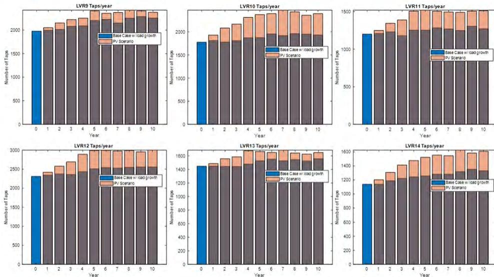
Figure 56: IEEE 123 PV1 - LVR operations per year with and without PV
