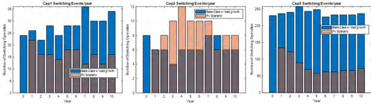
Figure 59: J1 - Capacitor switching per year - with and without PV
