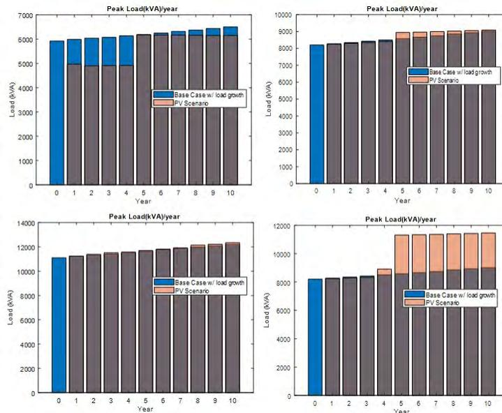
Figure 66: Feeder-wise yearly peak demand - with and without PV, Top Left: J1, Top Right: IEEE 123 PV, Bottom: IEEE 123 No PV
