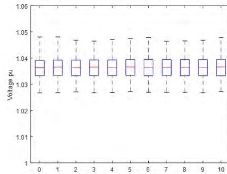
Minimum Circuit Voltage – No PV
