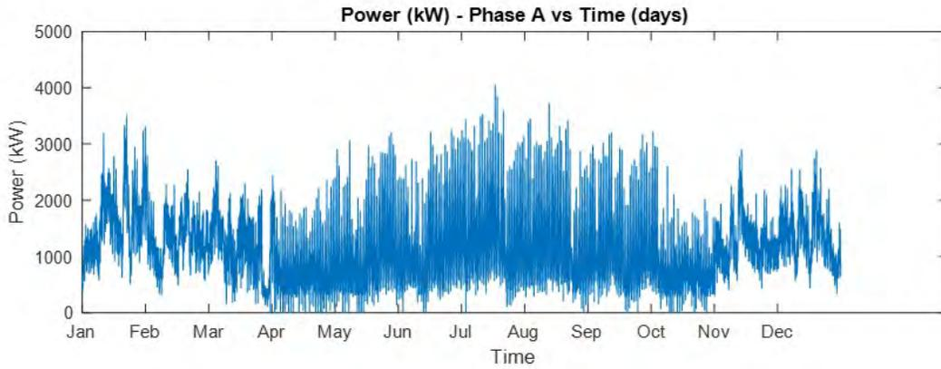
Figure 8: Net load at substation during year 10 - No PV
