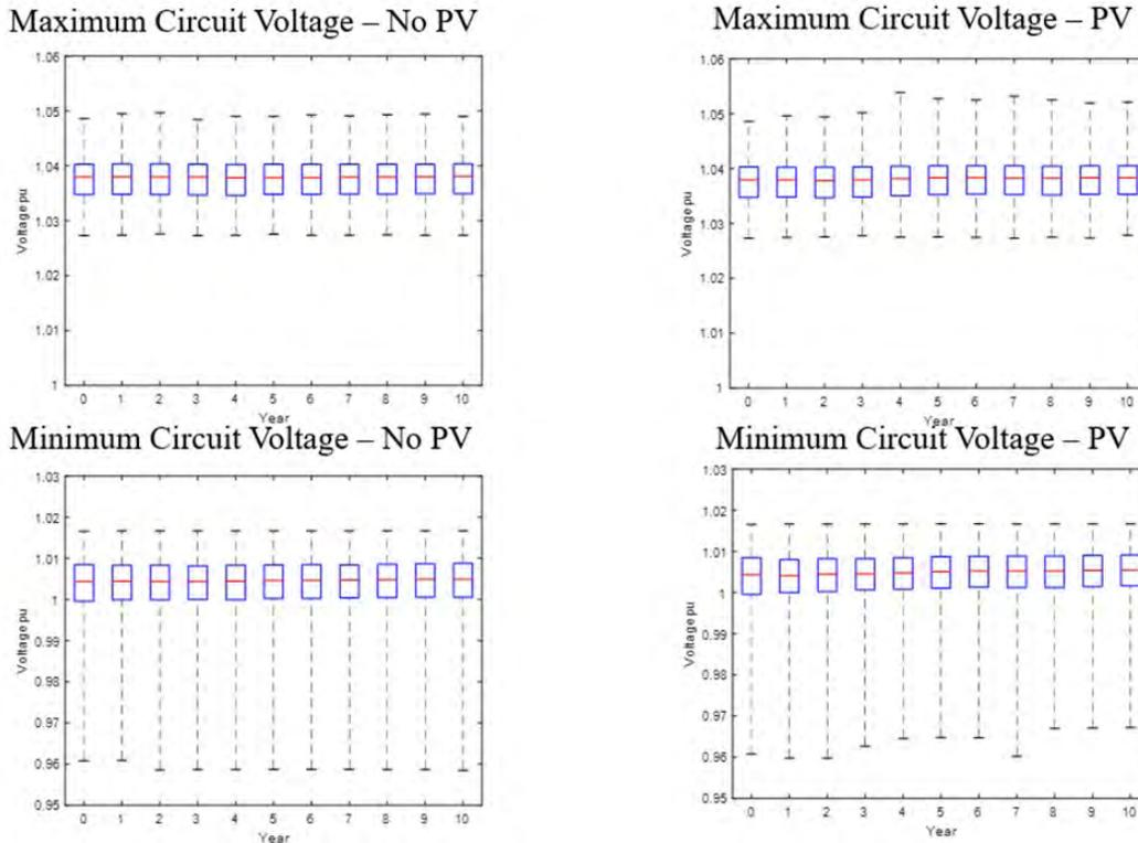
Figure 40: J1 - Voltage Statistics - with and without PV
