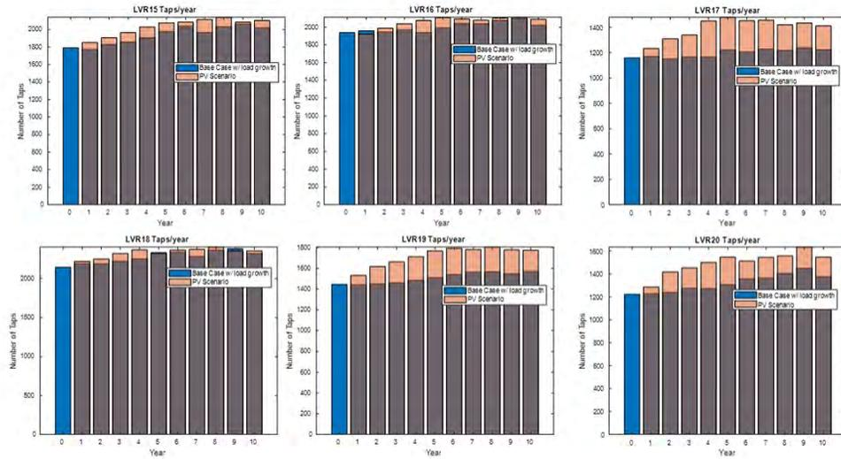
Figure 57: IEEE 123 No PV - LVR operations per year with and without PV
