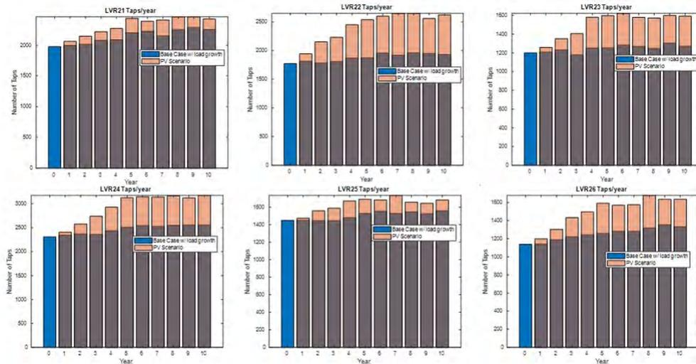
Figure 58: IEEE 123 PV2 - LVR operations per year with and without PV
