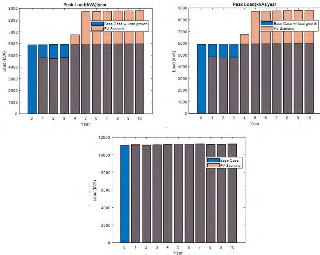
Figure 26: Feeder-wise yearly peak demand - with and without PV, Top Left: J1, Top Right: IEEE 123 PV, Bottom: IEEE 123 No PV
