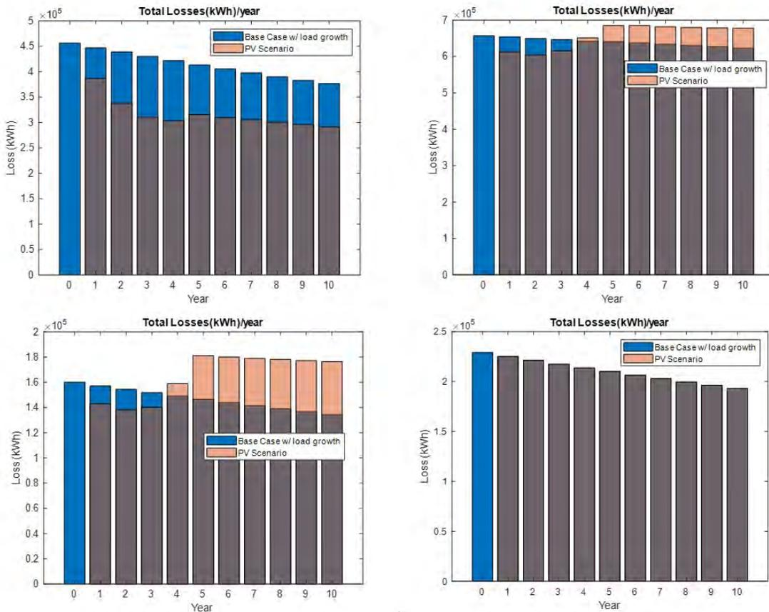
Figure 39: Feeder-wise losses per year - with and without PV, Top Left: Substation Area, Top Right: EPRI - J1, Bottom Left: IEEE 123 PV, Bottom Right: IEEE 123 No PV
