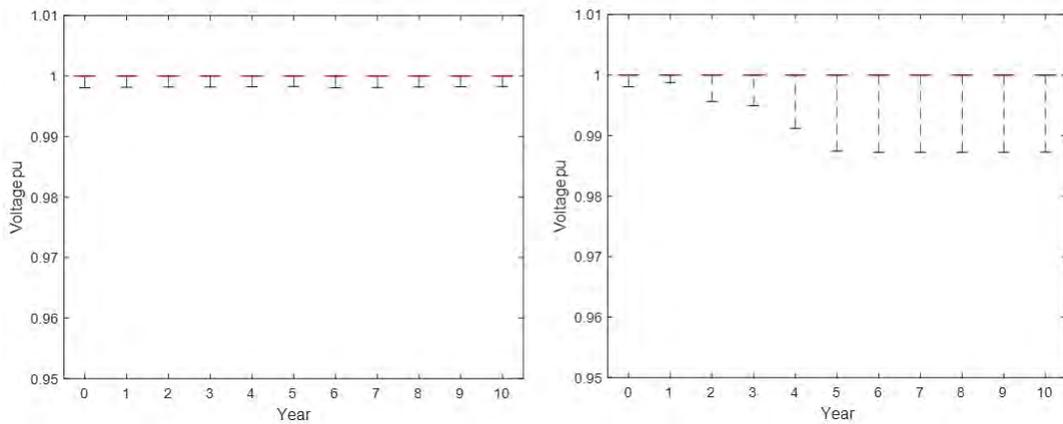
Figure 19: Minimum circuit voltage for each year of the planning period, Left: No PV, Right: with PV
