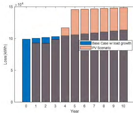
Figure 22: Yearly power loss in feeder - with and without PV
