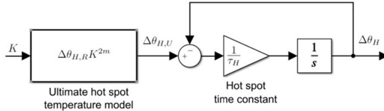
Figure A.3: The simulation model for hot spot temperature rise
