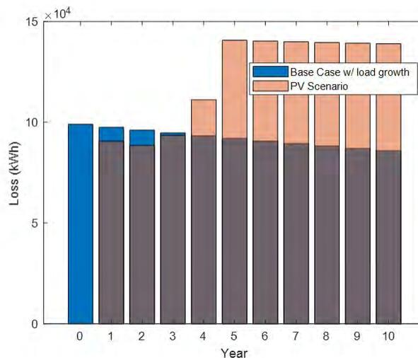
Figure 16: Total system losses per year - with and without PV
