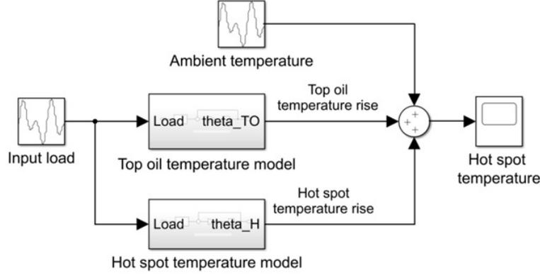
Figure A.1: Model for estimating the hot spot temperature of a transformer
