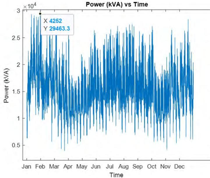
Figure 51: Net load profile year 10 - base case (No PV)
