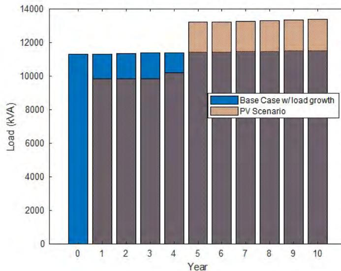
Figure 7: Yearly peak demand at the substation - with and without PV
