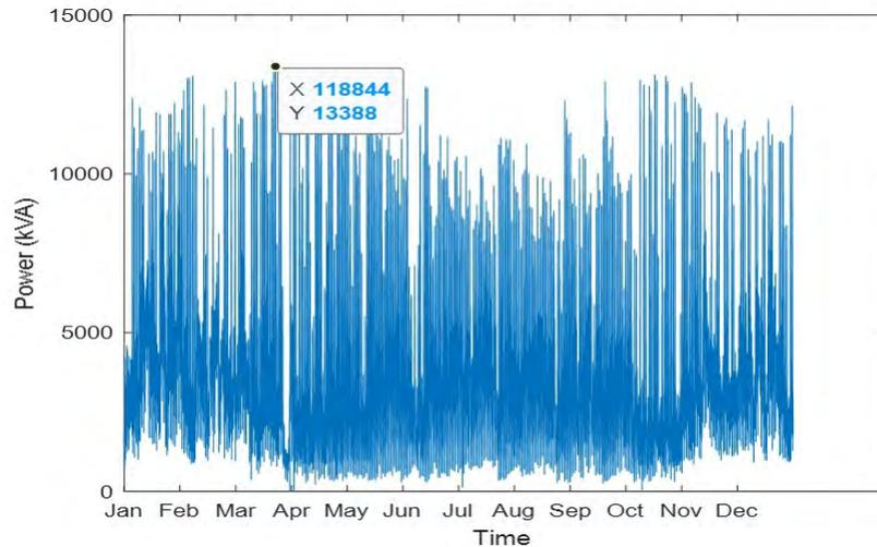
Figure 11: Net load profile during year 10 - with PV
