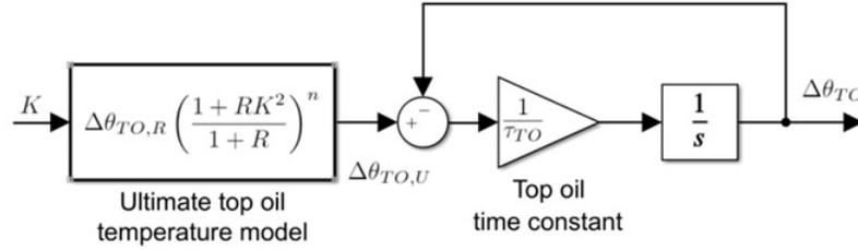
Figure A.2: The simulation model for top oil temperature rise
