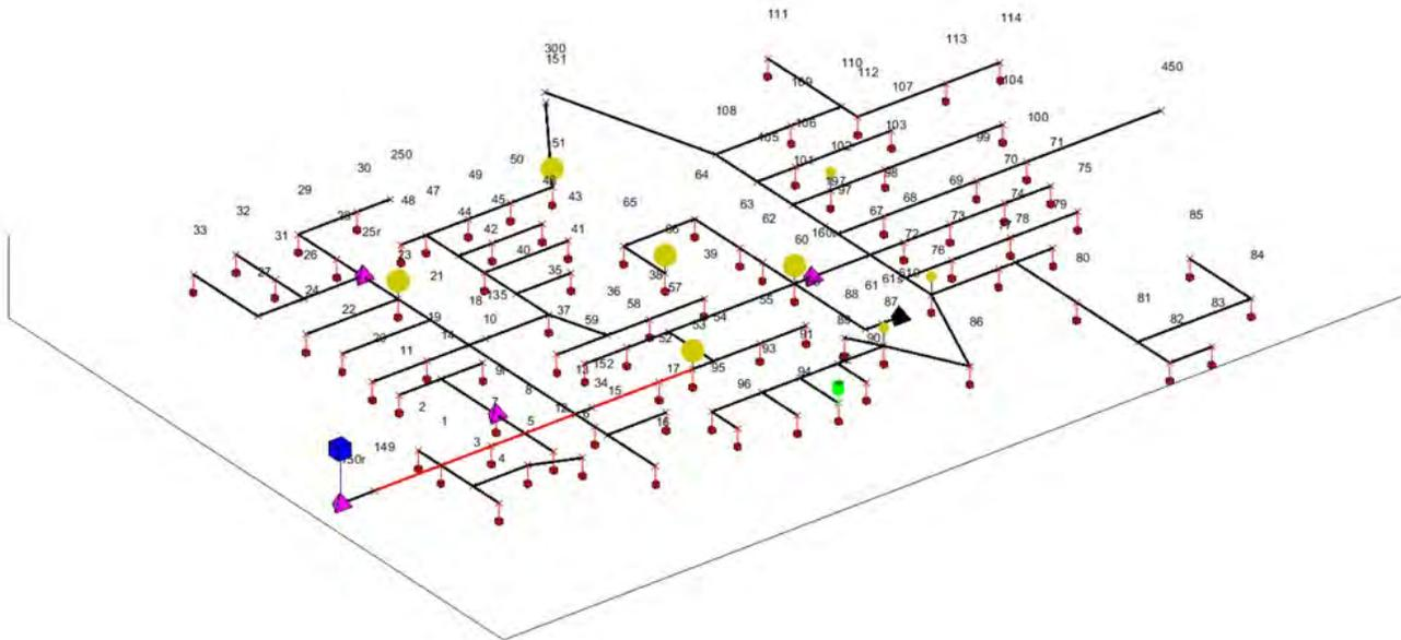
Figure 17: Equipment & line overloads in year 5 with PV
