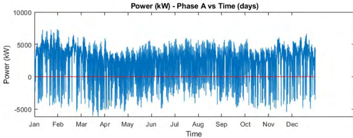
Figure 28: Net load at substation during year 10 with PV
