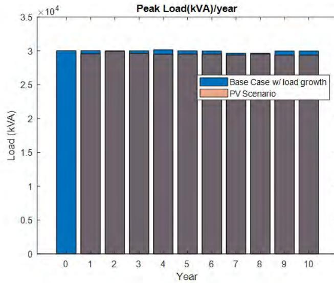
Figure 47: Yearly peak demand at substation - with and without PV
