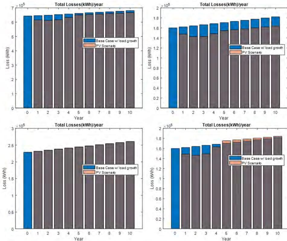
Figure 68: Feeder-wise total losses per year - with and without PV, Top Left: J1, Top Right: IEEE 123 PV1, Bottom Left: IEEE 123 No PV, Bottom Right: IEEE 123 PV2
