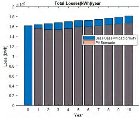
Figure 86: Total losses per year - with and without PV
