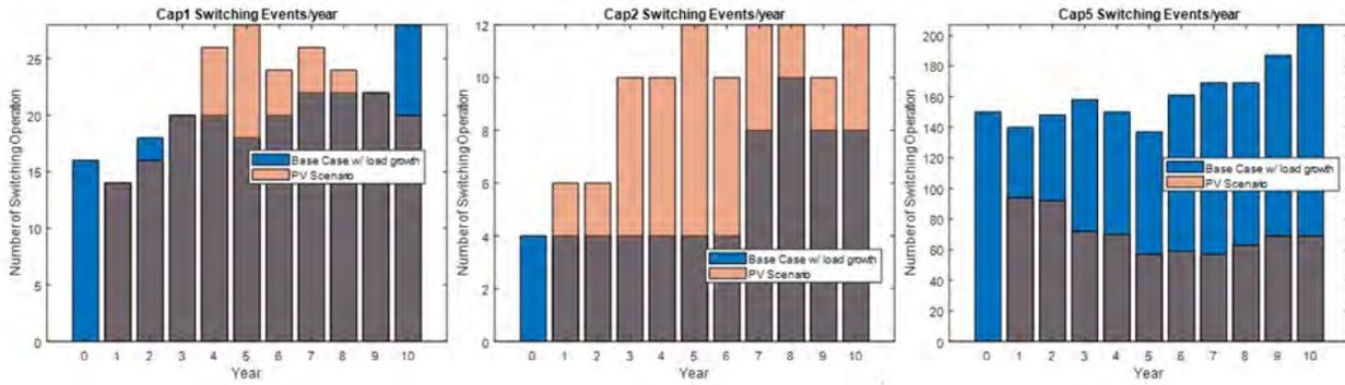
Figure 36: J1 - Capacitor switching per year - with and without PV
