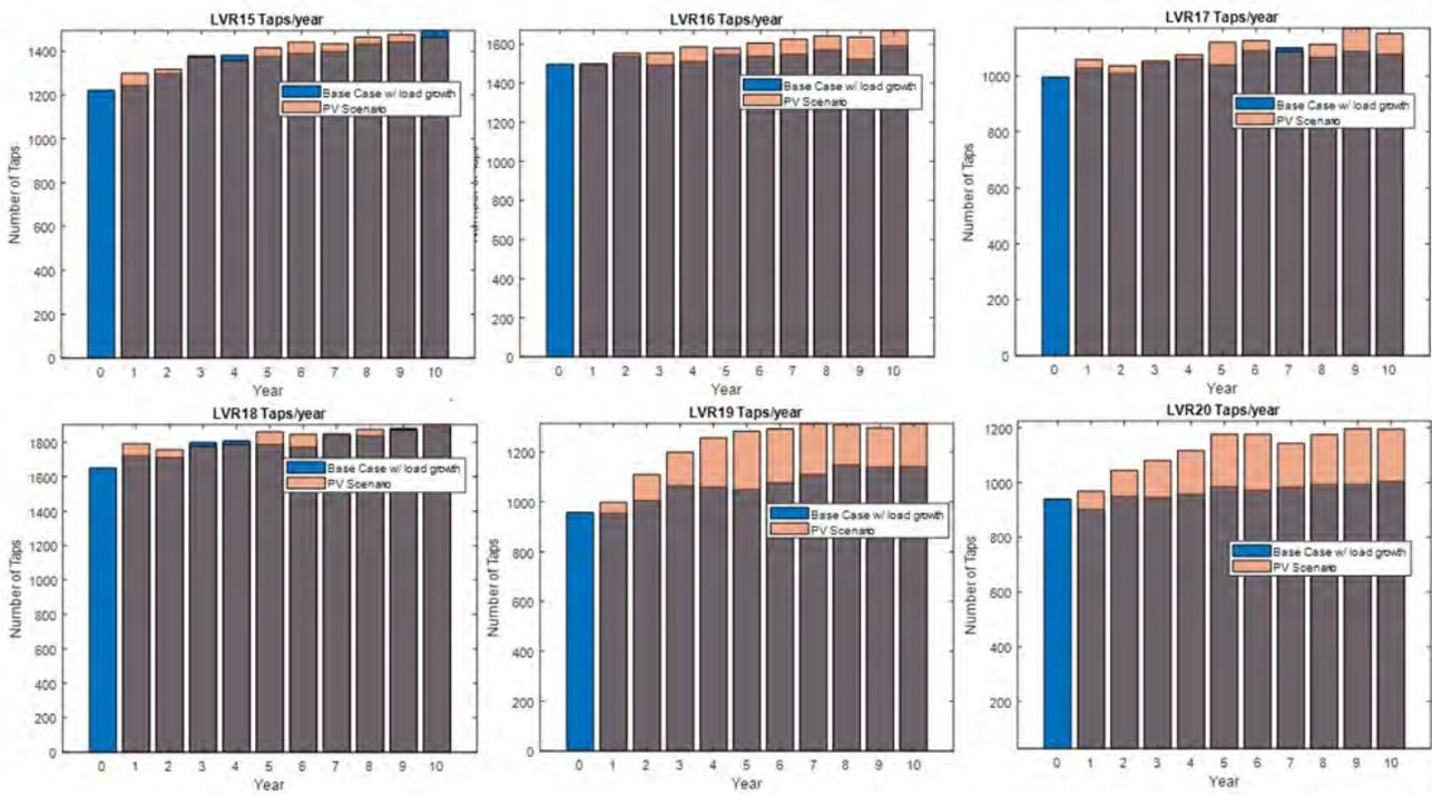
Figure 35: IEEE 123 No PV - LVR operations per year with and without PV
