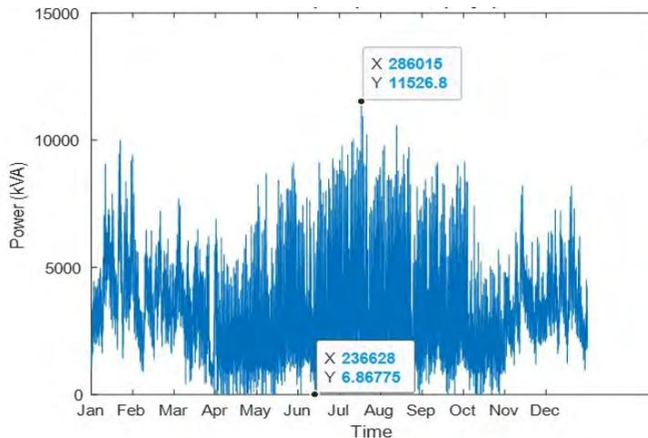
Figure 10: Net load profile during year 10 - base case (No PV)
