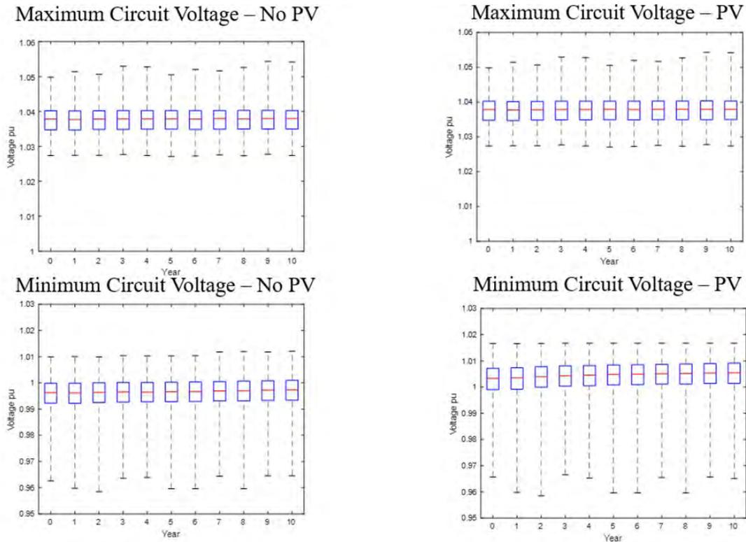
Figure 63: J1 - Voltage Statistics - with and without PV
