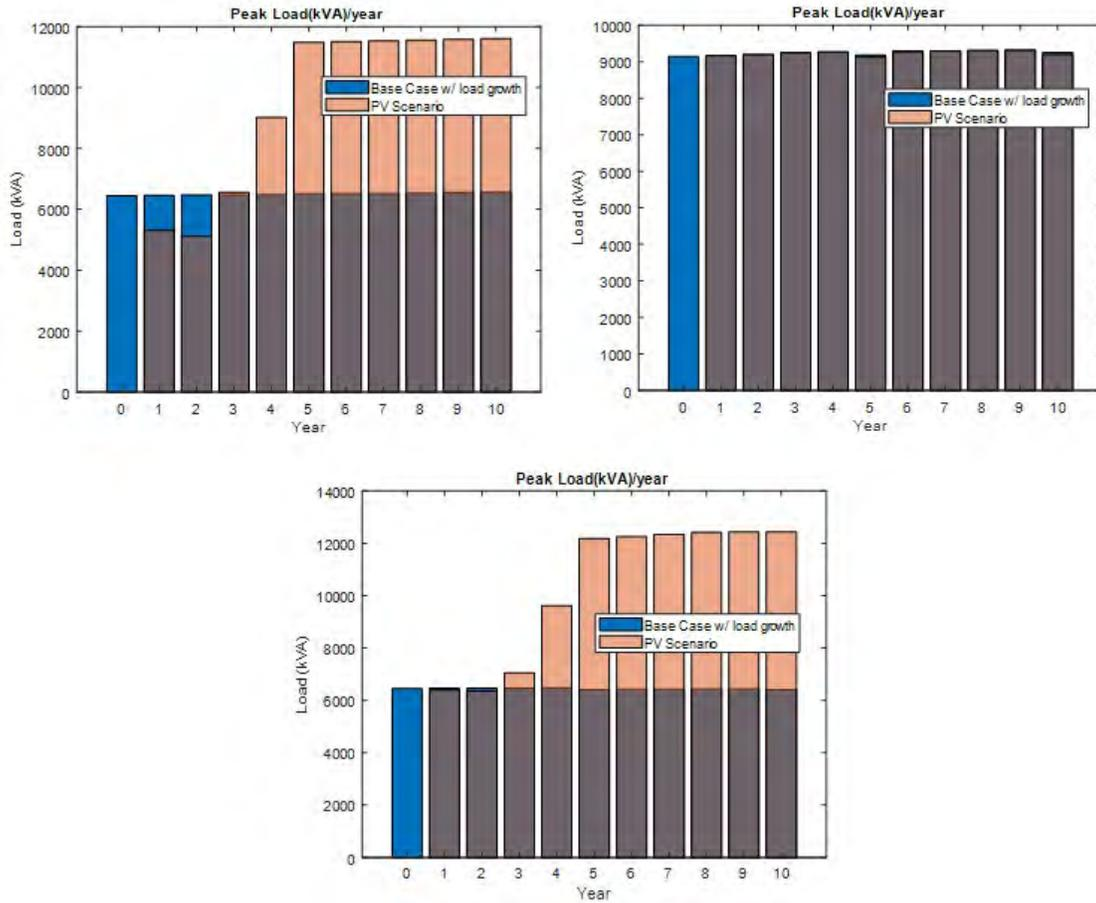
Figure 71: Feeder-wise yearly peak demand - with and without PV, Top Left: B01, Top Right: B02, Bottom: B03
