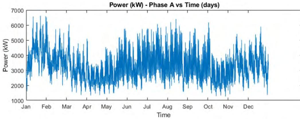
Figure 72: Net load at substation during year 10 without PV
