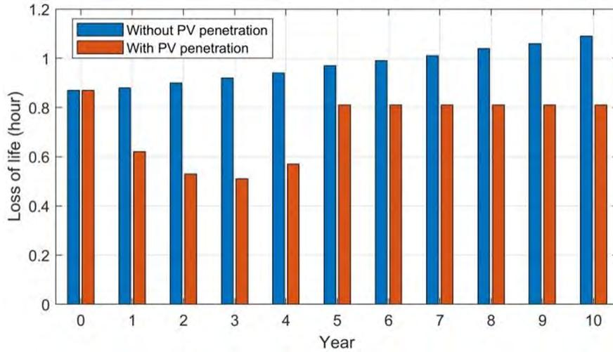
Figure 13: Comparison of transformer loss of life, with and without PV
