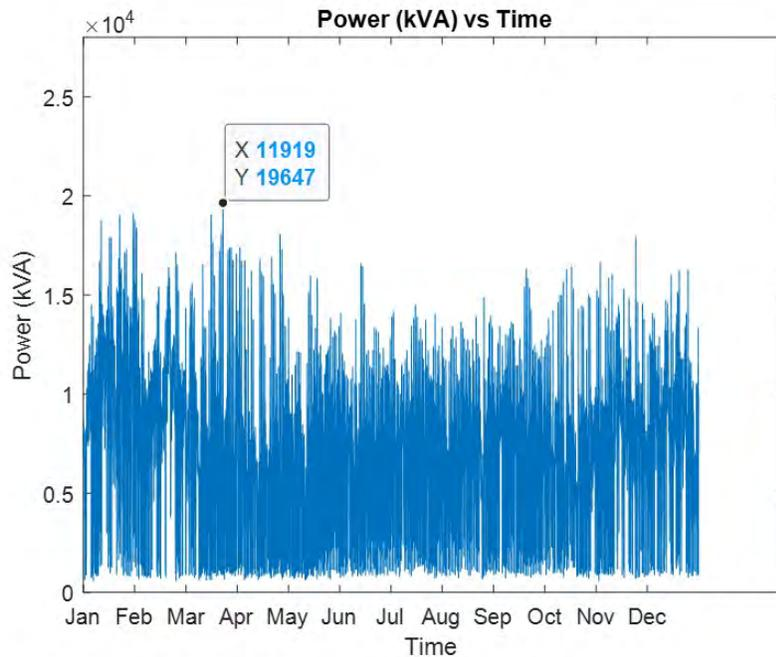
Figure 75: Net load profile year 10 - with PV
