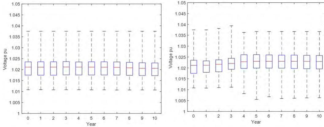
Figure 18: Maximum circuit voltage for each year of the planning period, Left: No PV, Right: with PV
