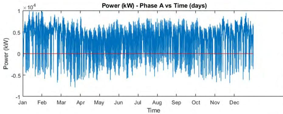
Figure 50: Net load at substation during year 10 with PV
