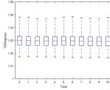
Minimum Circuit Voltage – No PV
