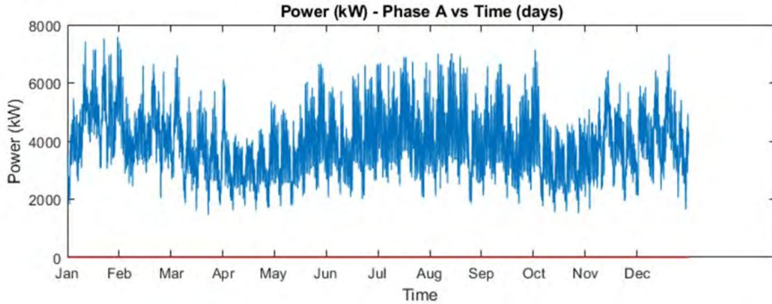
Figure 27: Net load at substation during year 10 without PV
