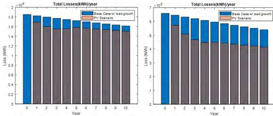
Figure 61: Total losses per year - with and without PV, Left: Total Distribution System, Right: Substation Area
