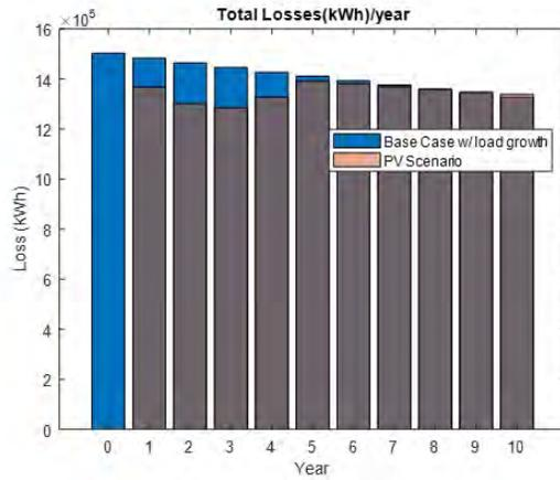
Figure 38: Total distribution system losses per year - with and without PV
