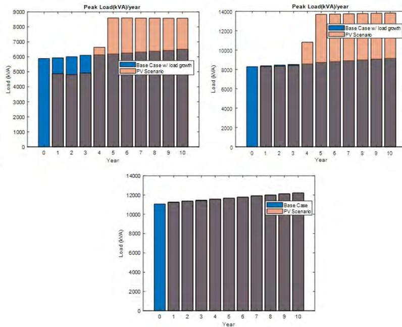
Figure 43: Feeder-wise yearly peak demand - with and without PV, Top Left: J1, Top Right: IEEE 123 PV, Bottom: IEEE 123 No PV
