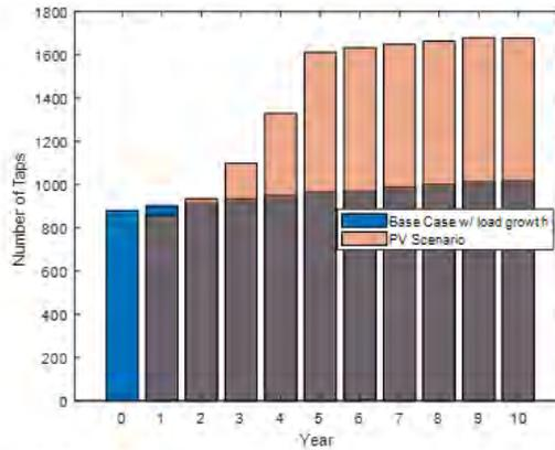
Increasing PV penetrations increases LTC operations and tapers off after year 5
