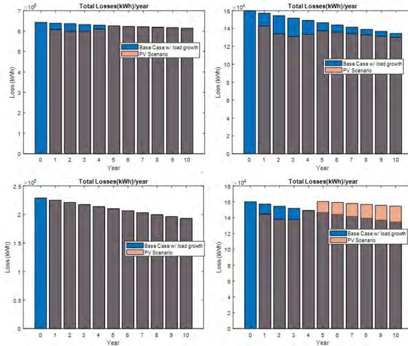
Figure 62: Feeder-wise losses per year - with and without PV, Top Left: J1, Top Right: IEEE 123 PV1, Bottom Left: IEEE 123 No PV, Bottom Right: IEEE 123 PV2
