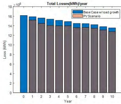
Figure 79: Total distribution system losses per year - with and without PV
