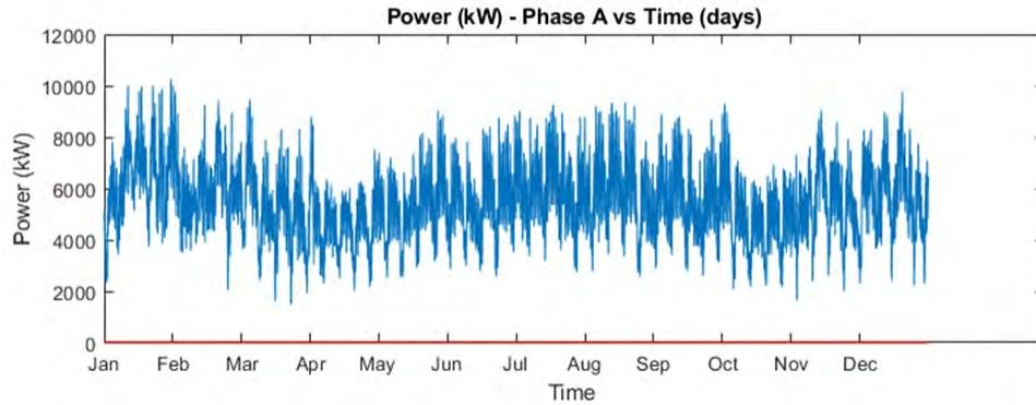
Figure 49: Net load at substation during year 10 without PV
