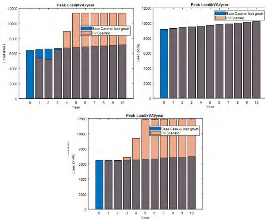
Figure 85: Feeder-wise yearly peak demand - with and without PV, Top Left: B01, Top Right: B02, Bottom: B03
