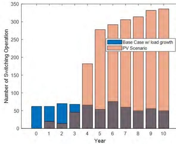
Figure 15: Capacitor switching per year - with and without PV
