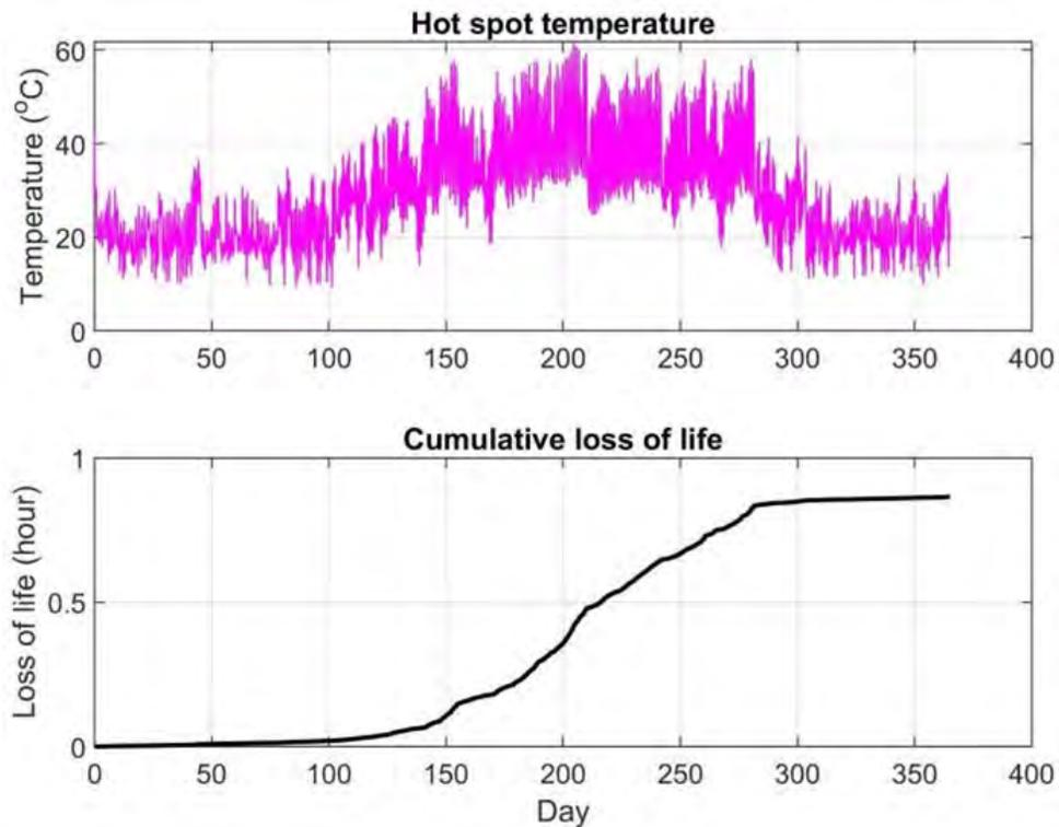
Figure A.6: Transformer hot spot temperature and loss of life
