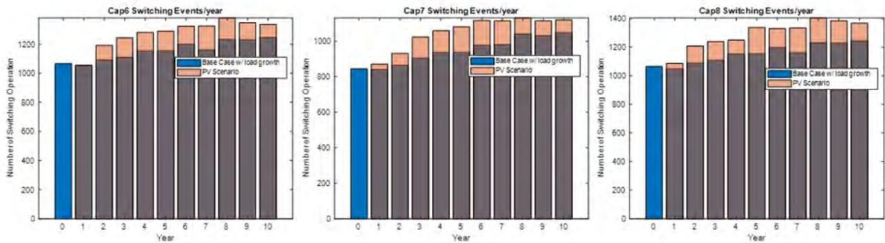
Figure 60: Capacitor switching per year - with and without PV - Left: IEEE 123 PV1, Middle: IEEE 123 No PV, Right: IEEE 123 PV2
