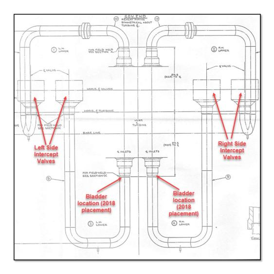
Figure 1: Turbine Steam Piping Diagram
