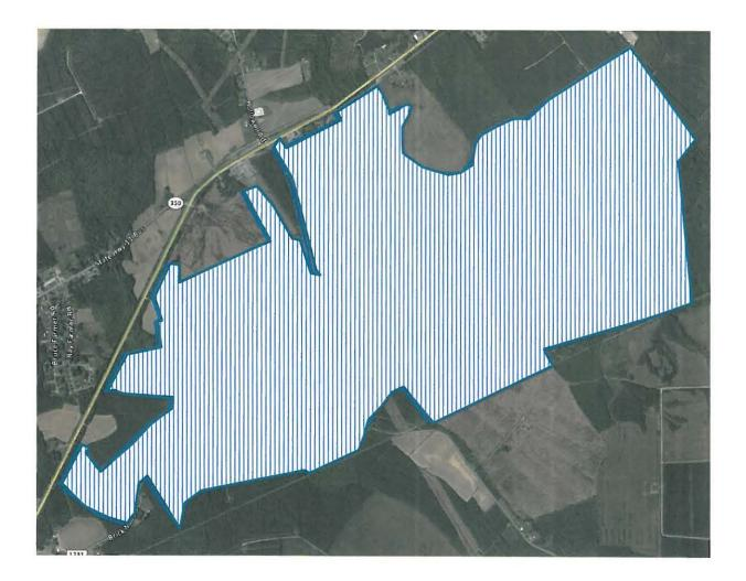
Outlined in BLUE above is the amended proposed layout that reflects the facility footprint. The blue diagonal lines depict modules and racking. No structures will be constructed on the site.
