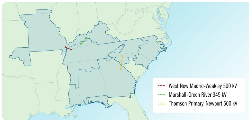
Figure L-6: SERTP Regional Analysis of Potential Transmission Project Alternatives
