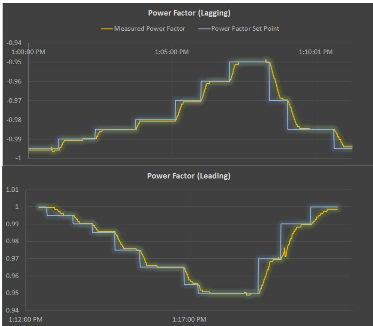
Figure 47. Lagging and leading power factor control tests. Illustration from First Solar
