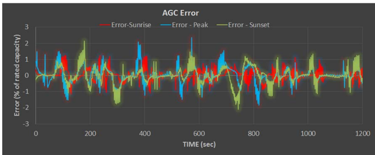
Figure 20. AGC control error for all three tests. Illustration from NREL
