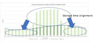
Next, the hypothetical illustration below shows an energy storage use case on the Companies' system as an overlay to the renewable energy production and the storage discharge times to see if there is alignment in charging and discharging periods between system operations
