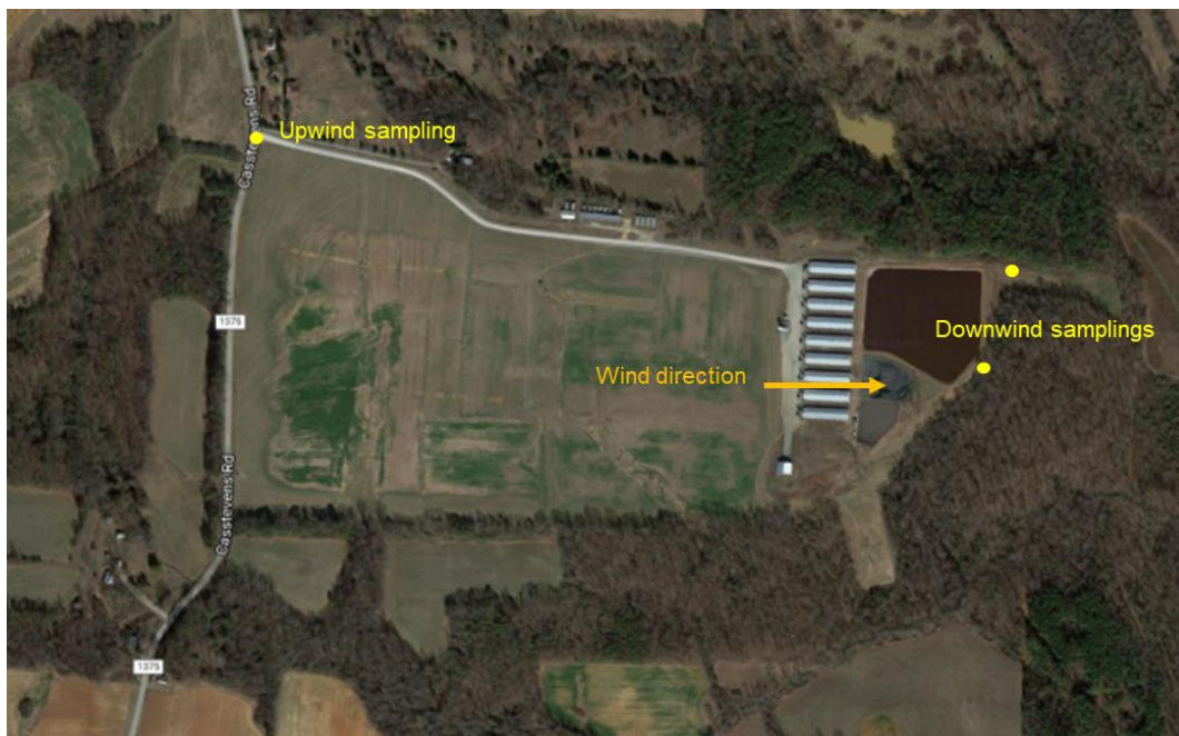
Figure 6. Aerial view of the facility and location of the monitoring points for odor for the December 31, 2019 sampling. The arrows indicate the prevailing wind direction the day of the sampling.
