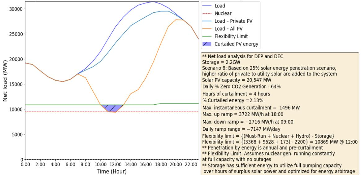
Fall Peak Net Load Day for 25% PV Penetration with higher ratio of private to utility solar added to the system
