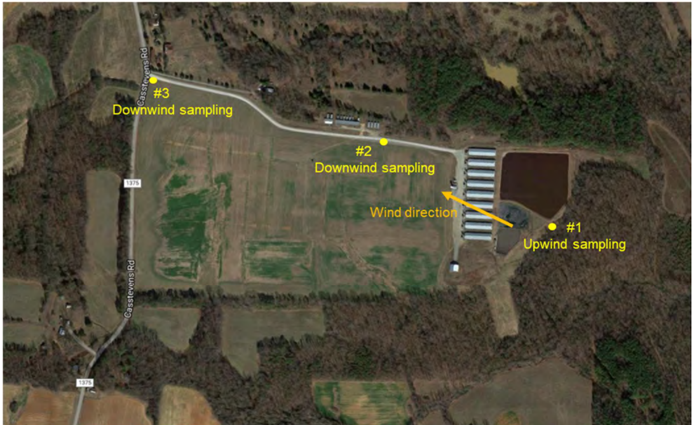
Figure 4. Aerial view of the facility and location of the monitoring points for odor for the June 26, 2018 sampling. The arrows indicate the prevailing wind direction the day of the sampling.
