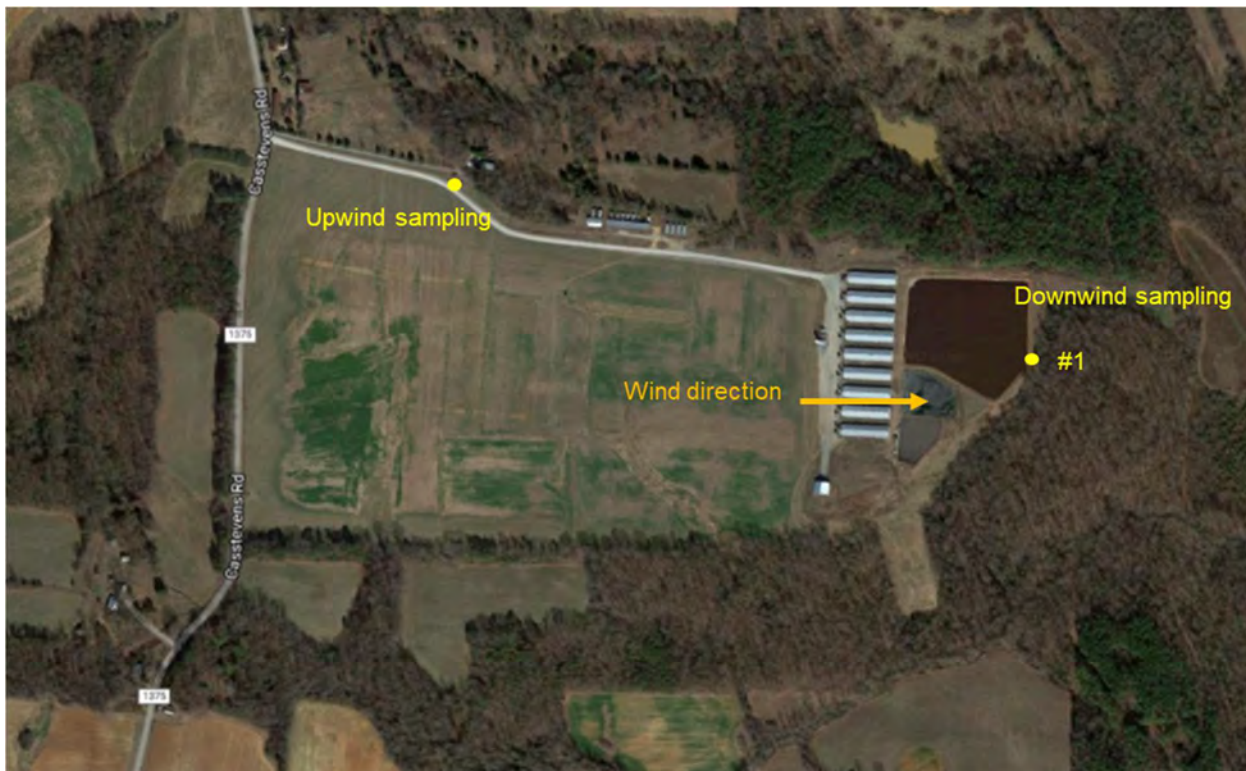
Figure 5. Aerial view of the facility and location of the monitoring points for odor for the June 26, 2018 sampling. The arrows indicate the prevailing wind direction the day of the sampling.
